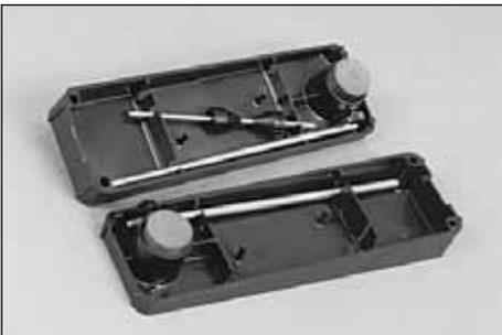
• Place all components into the case halves in the positions shown in the photo. Press on the **ends** of the rods (not in the middle) when storing, to prevent bending. We recommend storing one base rod in each case half, for minimum case distortion.
