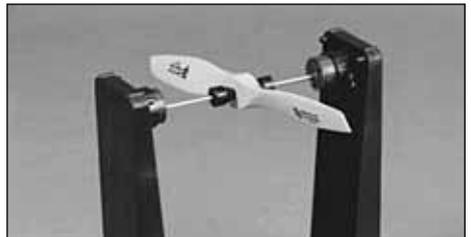
**How to balance SMALL AND MEDIUM SIZE PROPELLERS:** Slide the cones onto the balancer shaft with the tapered ends facing each other, trapping the propeller between the cones. The object
